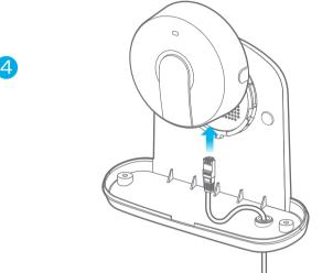
(a) S Attach the AP to the inner case by rotating it in a clockwise direction until it clicks into place.
