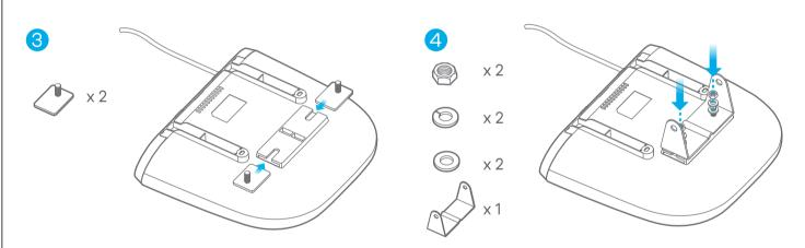
(a) S Align the rotating bracket's holes with the holes on the M-type bracket.
